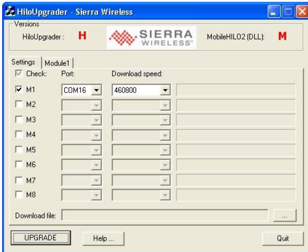
Figure 2 HiloUpgrader Graphical User Interface. H gives the version of HiloUpgrader, M the version of MobileHilo2 DLL.
